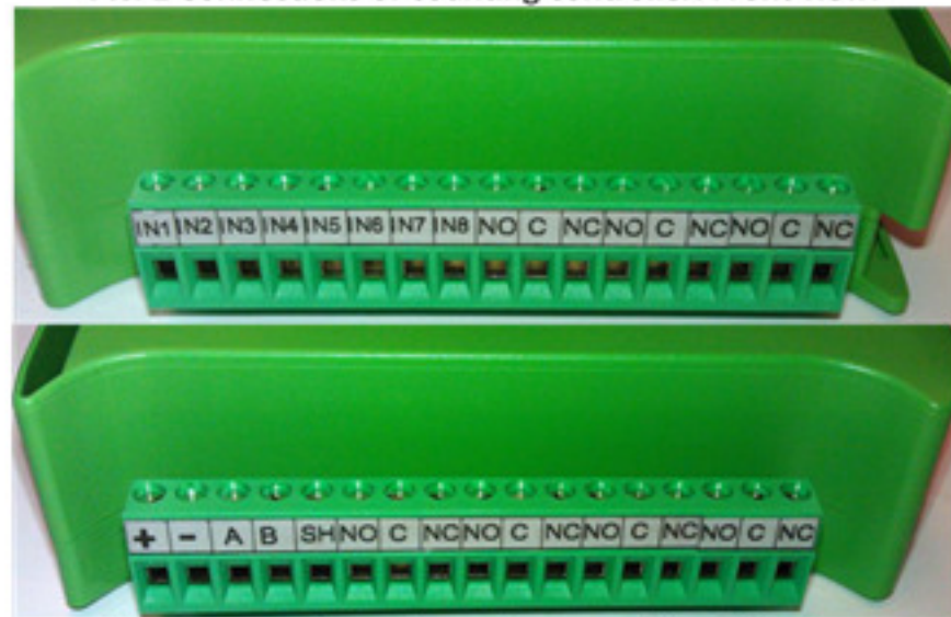
Pic. 3 Connections of counting controller. Side view.
