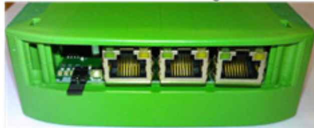
Pic. 2 Connections of counting controller. Front view.
